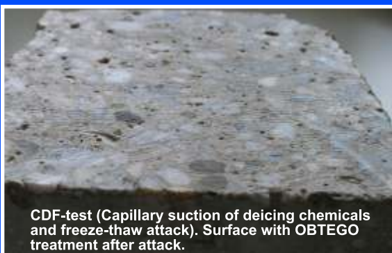
CDF-test (Capillary suction of deicing chemicals and freeze-thaw attack). Testing method of frost and deicing salt resistance on concrete.
